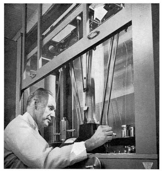
WEIGHING A VESSEL AND ITS VALVES on analytical balance is part of process metrology technician Chuck Shinneman (8112-1) uses to determine the volume - to an accuracy of  $\pm$  2 milligrams — of the vessel. Increasing the accuracy of the balance from  $\pm$  15 milligrams to ± 2 milligrams resulted from installation of a photoelectric tilt indicator (arrows) designed jointly by Chuck and electronics technician Mike Rogers (8151).
